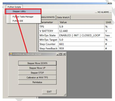
From this window you will have full control of the stepper actuator. You can move the stepper DOWN and UP or you can STOP it.
