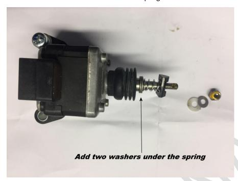
The BOLT for stepper command lock, must be opened (calibration is then possible using STEPPER.PY python script), and then it must be fixed with Loctite, see next page for details:
