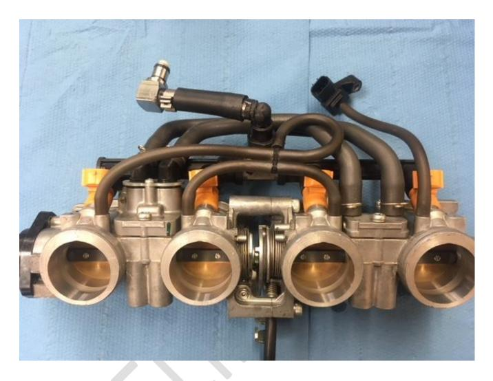
Finally MAP sensor must only be connected to Cylinder 4, and cylinders 1,2 and 3 must be connected together through the hoses.
